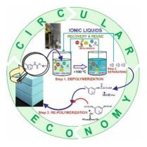
**Figure 1**. Schematic representation of the depolymerization process of polyurethane foam waste, including recovery and reuse of polyols.
